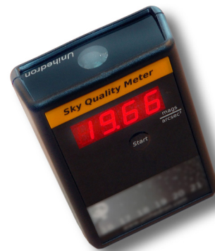
Image 25. A sky quality meter (SQM) is an instrument used to measure light pollution from the ground. Image: Lamiot / CC BY-SA ( https://creativecommons.org/licenses/by-sa/3.0 )
